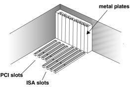
Figure 1. Locating a PCI slot
